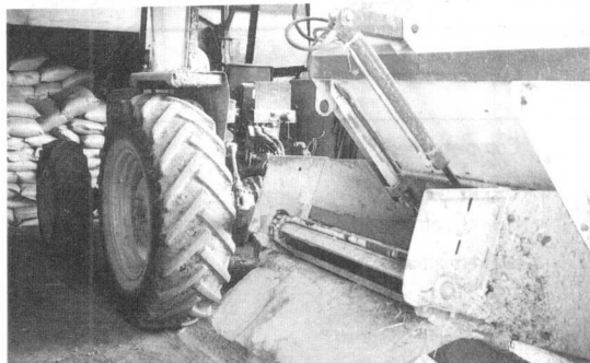
Fig. 5. An outside opening of mixer for the direct feeding of total mixed ration.
