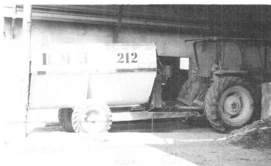
Fig. 3. T.M.R. mixer with coupling device for operating power
